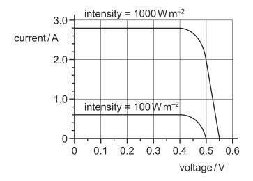
current at 1000 W m<sup>-2</sup> At zero voltage, what is the ratio current at 100 W m<sup>-2</sup>
