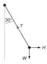
The tension in the string of the pendulum is T. The weight of the pendulum bob is W.
