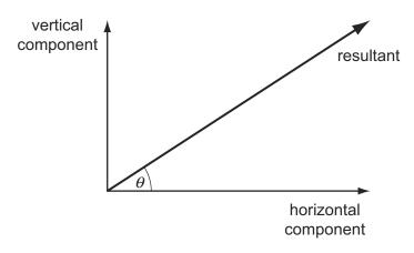
The horizontal component is 20.0 N and  $\theta$  = 30°. What is the vertical component?
